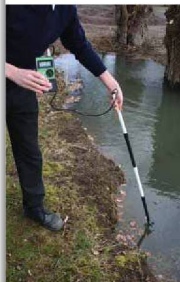
▲ A flow-meter allows water velocity to be recorded at any depth.
